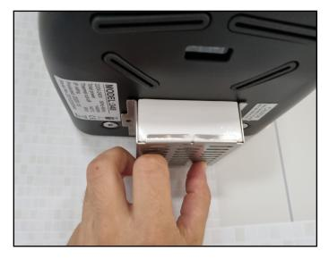
2. Place the filter unit on the holes over the air inlet.
