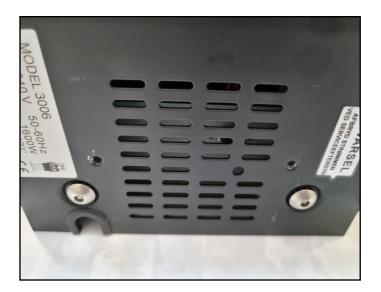
1. Locate the mounting holes on the foot of the dryer. Remove existing filter holder, if any, before the new unit can be installed.
