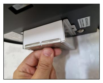
2. Place the filter unit on the holes over the air inlet.
